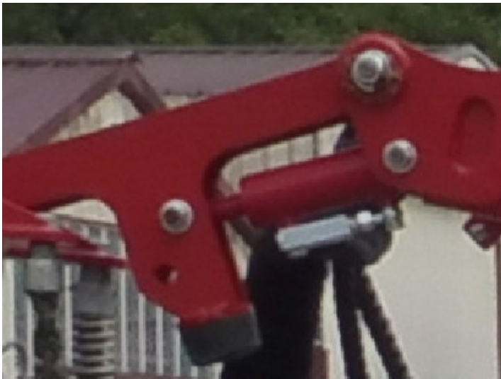
Adjustment of the «wrist» by hydraulic cylinder
