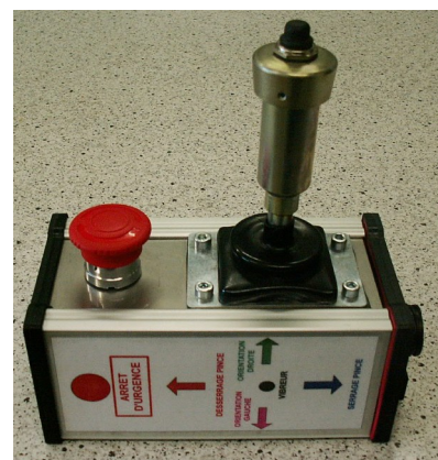
ELECTRICAL CONTROL ASSEMBLED IN THE DRIVER'S CAB
